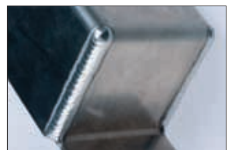
Welding of thin Aluminium with AC TIG
